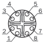
Figure 7: Female connector, M12, 8-pin, X-coded
